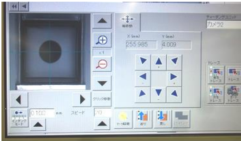
Figure 4: Yamaha YS mounter's pick-up nozzle positioning screen (Reference)
